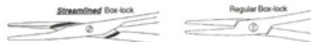
Streamlined needle holders feature a smooth (streamlined) box-lock that does not snag suture when tying.
