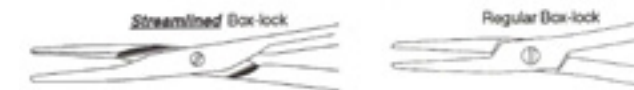
Streamlined needle holders feature a smooth (streamlined) box-lock that does not snag suture when tying.
